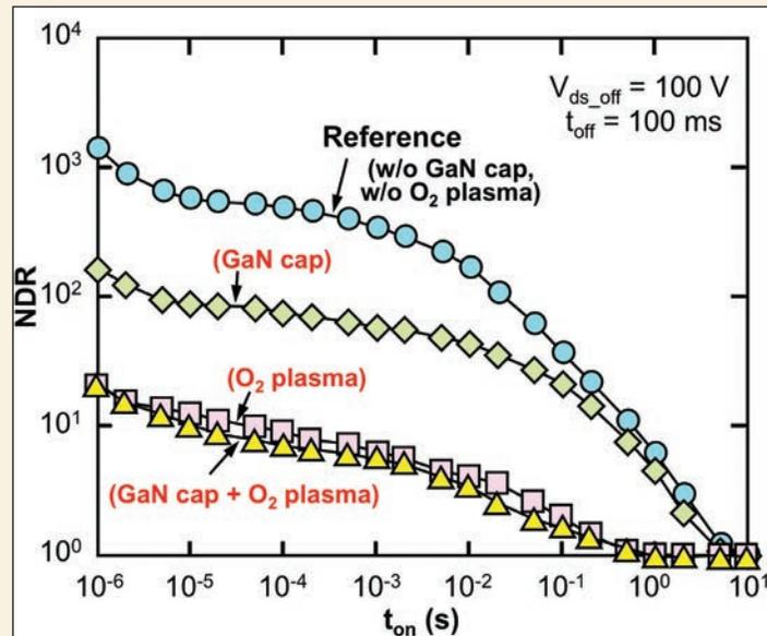
Oxygen plasma treatment is a very effective way to reduce current-collapse, which has been evaluated by considering the ratio of dynamic on-resistance to static on-resistance.
